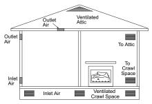
Figure 3 - Ventilation Air from Outdoors
